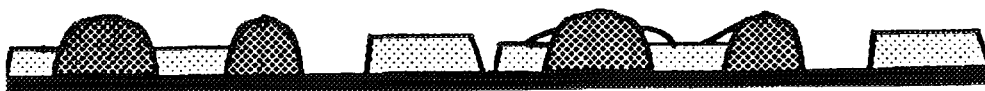
FIG. 6. Microstructure of Rh/Ce on SiO 2 after treatments indicated. Rh particles are dispersed on the thick Ce island structure by heating in NO. Some Rh is volatilized by heating in NO + CO, as evidenced by the absence of Rh particles after reduction.
